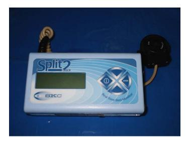
The real time dust monitor provided the  $PM_{10}$  data. The complete data records are available in electronic format at the civil engineering department, LAU.
